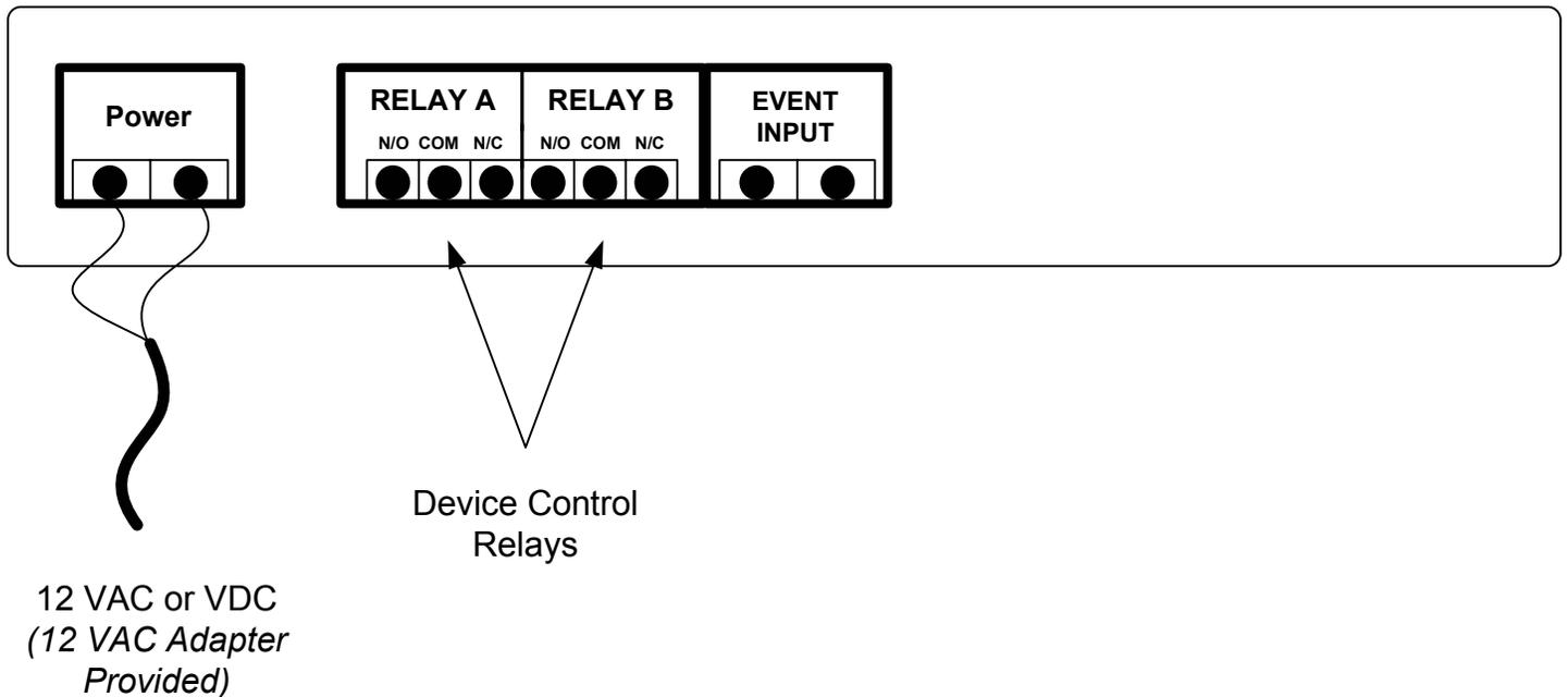
This diagram show the basic hook-ups for the remote sytation (“gatebox”). Installation is common to most keypad installations. You need two wires for power and two wires for device (“gate”) control.
